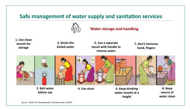
In places where centralized water treatment and safe piped water supplies are not available, a number of household water treatment technologies are effective in removing or destroying viruses as shown in the figures.
