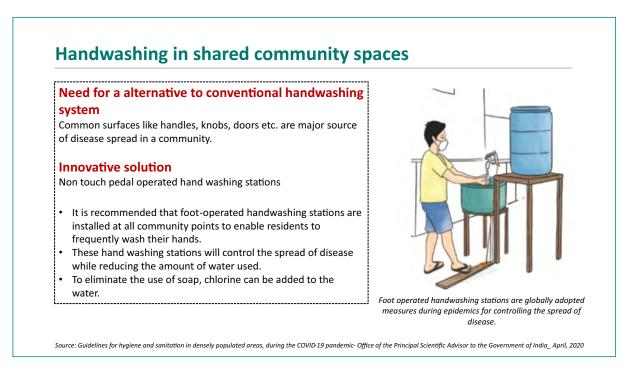
The spread of the virus is mainly through hands hence alternative systems to conventional handwashing are recommended. Pedal operated handwashing facilities are suggested to be installed in communities with shared facilities to enable handwashing without touching the taps by hands. Innovative solutions for different techniques should be encouraged.
