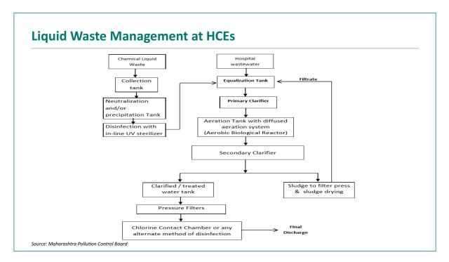
Waste water from COVID-19 hospitals to be disinfected with primary treatment and then treated in STP to meet discharge standards including chlorination.
