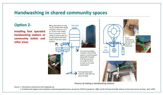
As suggested in 'Guidelines for hygiene and sanitation in densely populated areas during COVID-19 pandemic' by GoI, simple mechanisms can be used for installation of foot operated handwashing stations. These mechanisms can be developed by using lever, brakes wires, etc.
