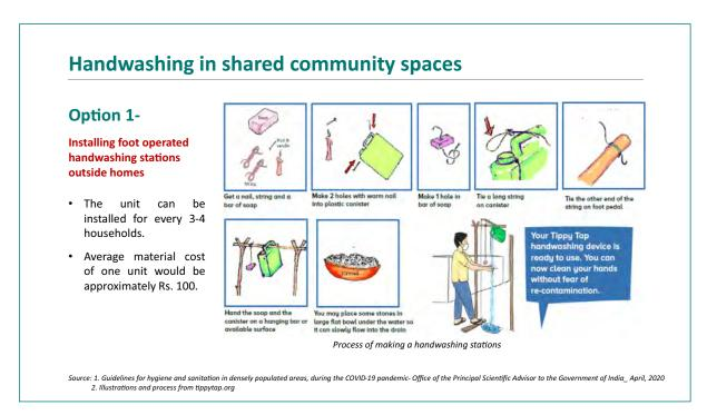
For smaller scale of ULBs, it is advisable to go for low cost technique of pedal operation which can be quickly installed in communities for use. It should be ensured that the material used should be available easily.
