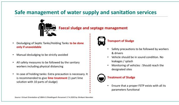
Desludging of septic tanks and transportation of sludge can prove fatal if necessary precautions are not taken and hence need to be monitored closely. Manual desludging should be strictly prohibited. Vehicles for transportation should be well maintained and regularly disinfected. Operation and maintenance of FSTPs should be done by monitoring all parameters.
